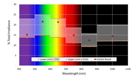
400-500 nm = 15.1774% Class A 500-600 21.5593% Class A nm = Class A 600-700 21.3764% nm = Class A 700-800 nm = 14.9445% 800-900 nm = 12.4609% Class A 900-1100 nm = 14.4815% Class A
